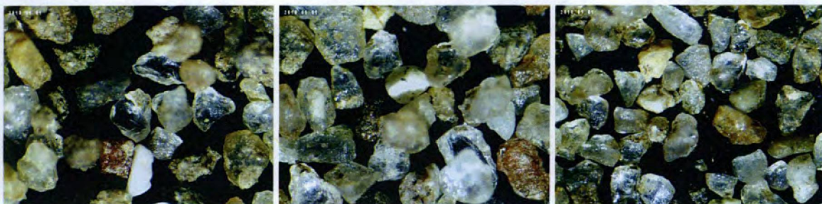
Figure 4: Waypoint 11, Potential Product Pictures – Samples washed using simulated attrition method (70% solids by weight, 2 minutes, x4 magnification)
