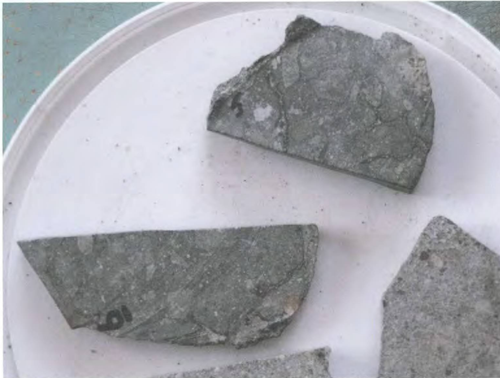
ONLY A SMALL AMOUNT OF VERY FINE MATERIAL SLOUGHED FROM THE REGULAR WATER FREEZE/THAW
