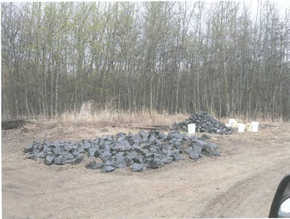
SAMPLE OF LARGER PIECES LAID OUT FOR WEATHERING TEST
