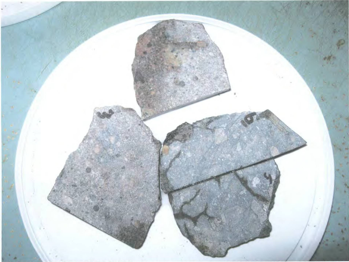
SLABS DRYING AFTER A FREEZE/THAW TEST SHOWING FRACTURES HOLDING WATER LINKED TO THE GREEN VOLCANIC ROCK
