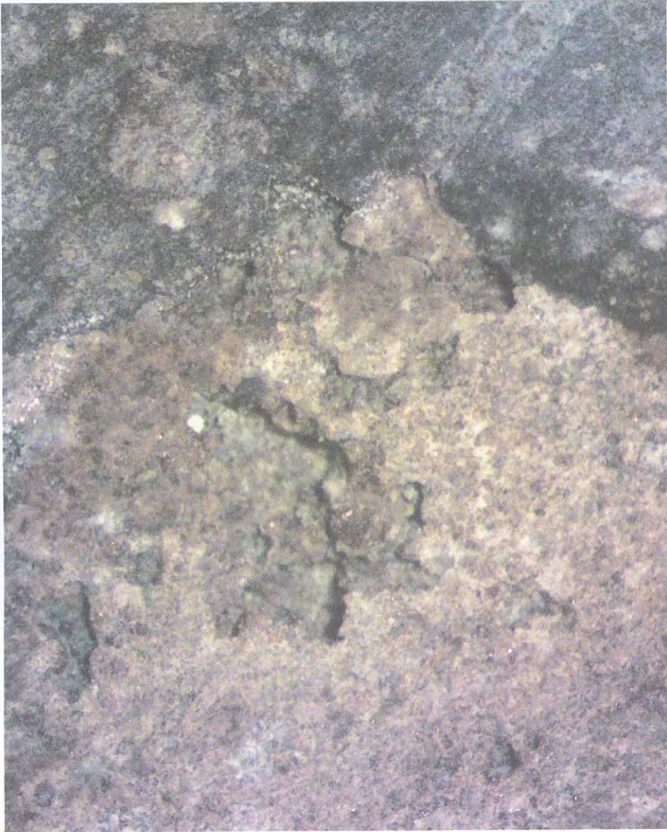
Very rare pop-outs in green rock from fresh water freeze thaw
