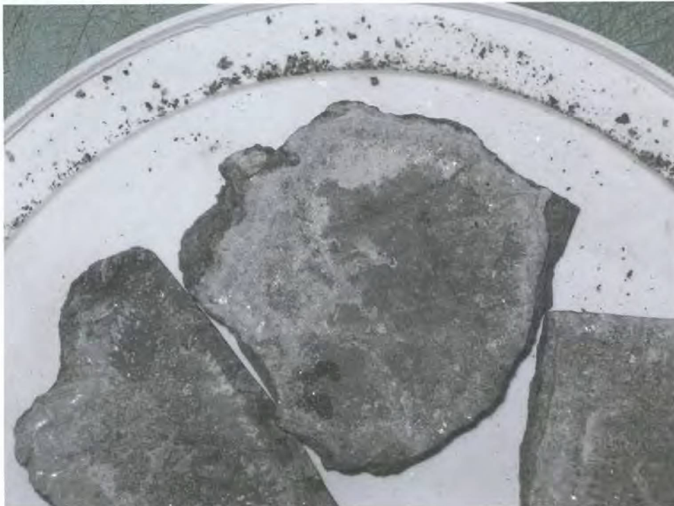
FINE GRAINED MATERIAL SLOUGHED OFF THE SLABS DURING SALTED FREEZE/THAW
