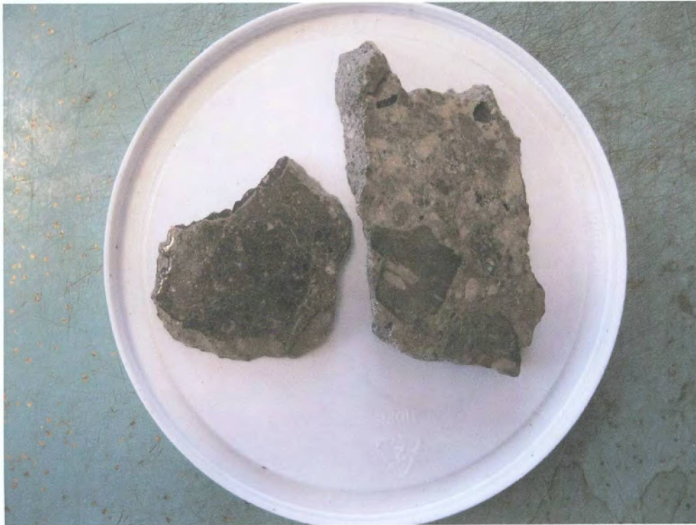
RESIN COATED SAMPLES SHOWING COATED FACE
