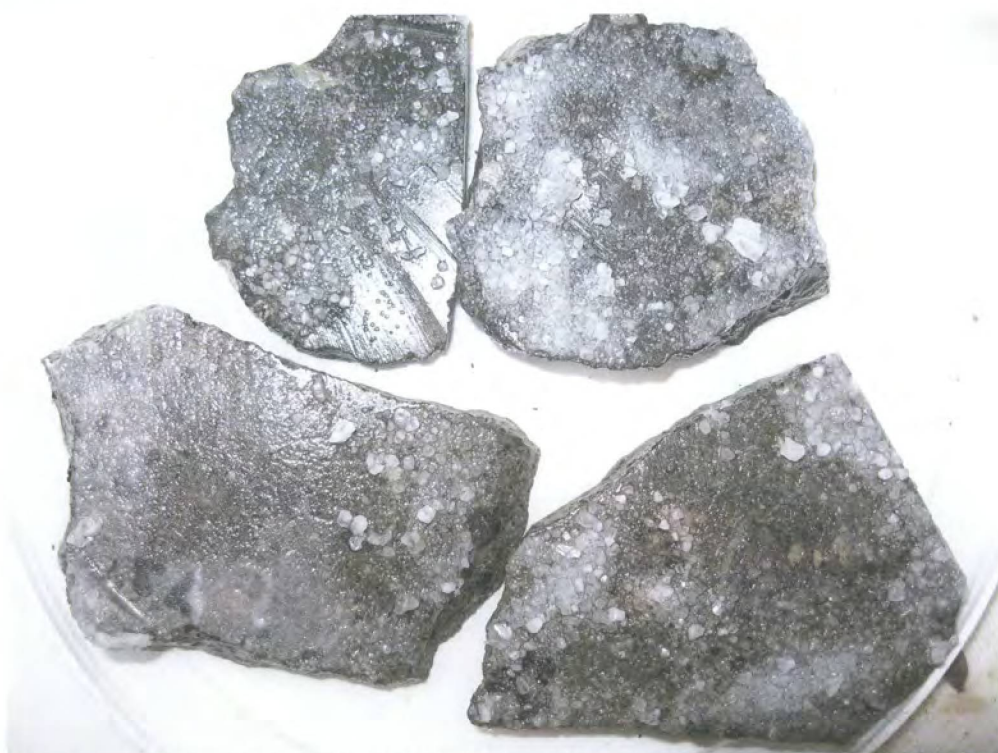
SALTED SAMPLES IN FREEZE/THAW SHOW A WET LOOK AS WATER CONTINUES TO COME OUT OF THE SALT AS THE SAMPLE DRIES
