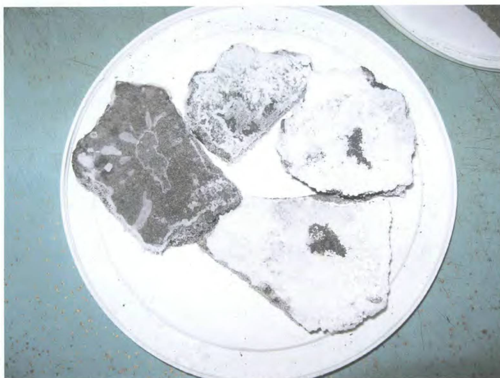
WHEN FULLY DRY THE SALTED FREEZE/THAW SAMPLES SHOW DEFINITE SALT CRUST
