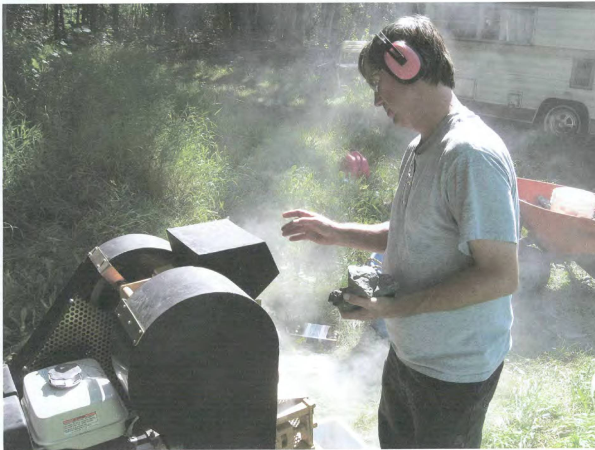
TESTING SAMPLES IN A 4 X 6 INCH JAW CRUSHER
