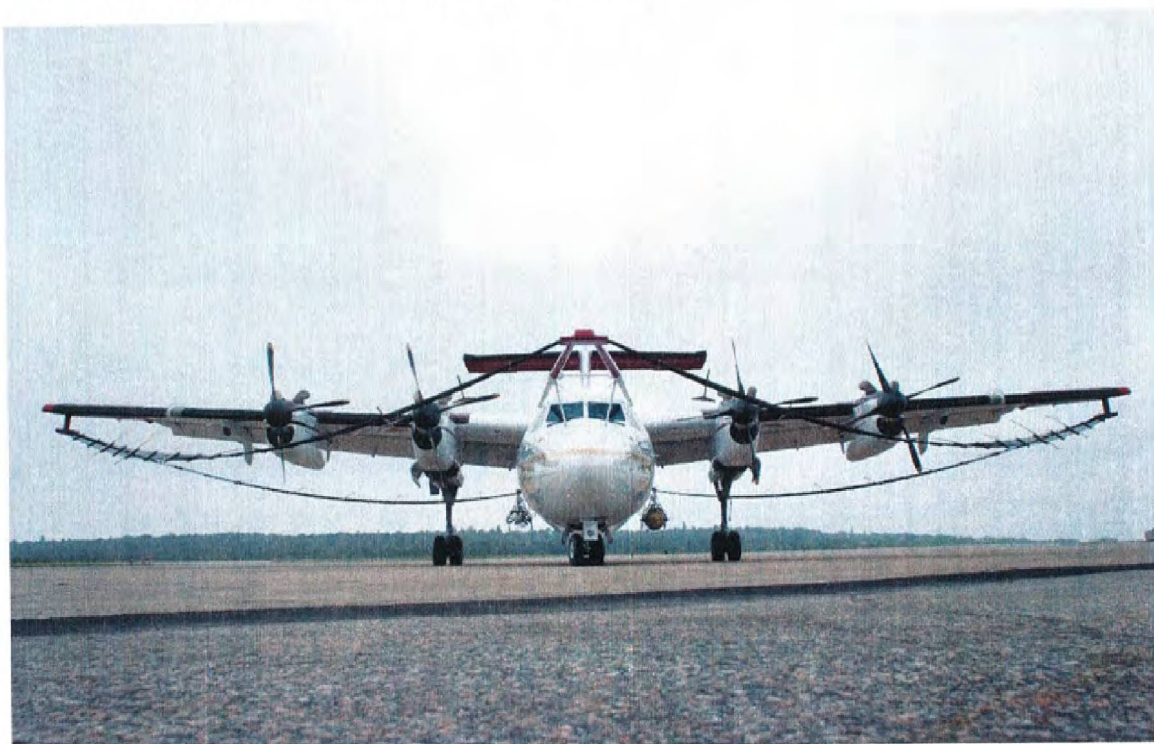
Figure 1: Specially modified Dash-7 aircraft used by Fugro Airborne Surveys.
