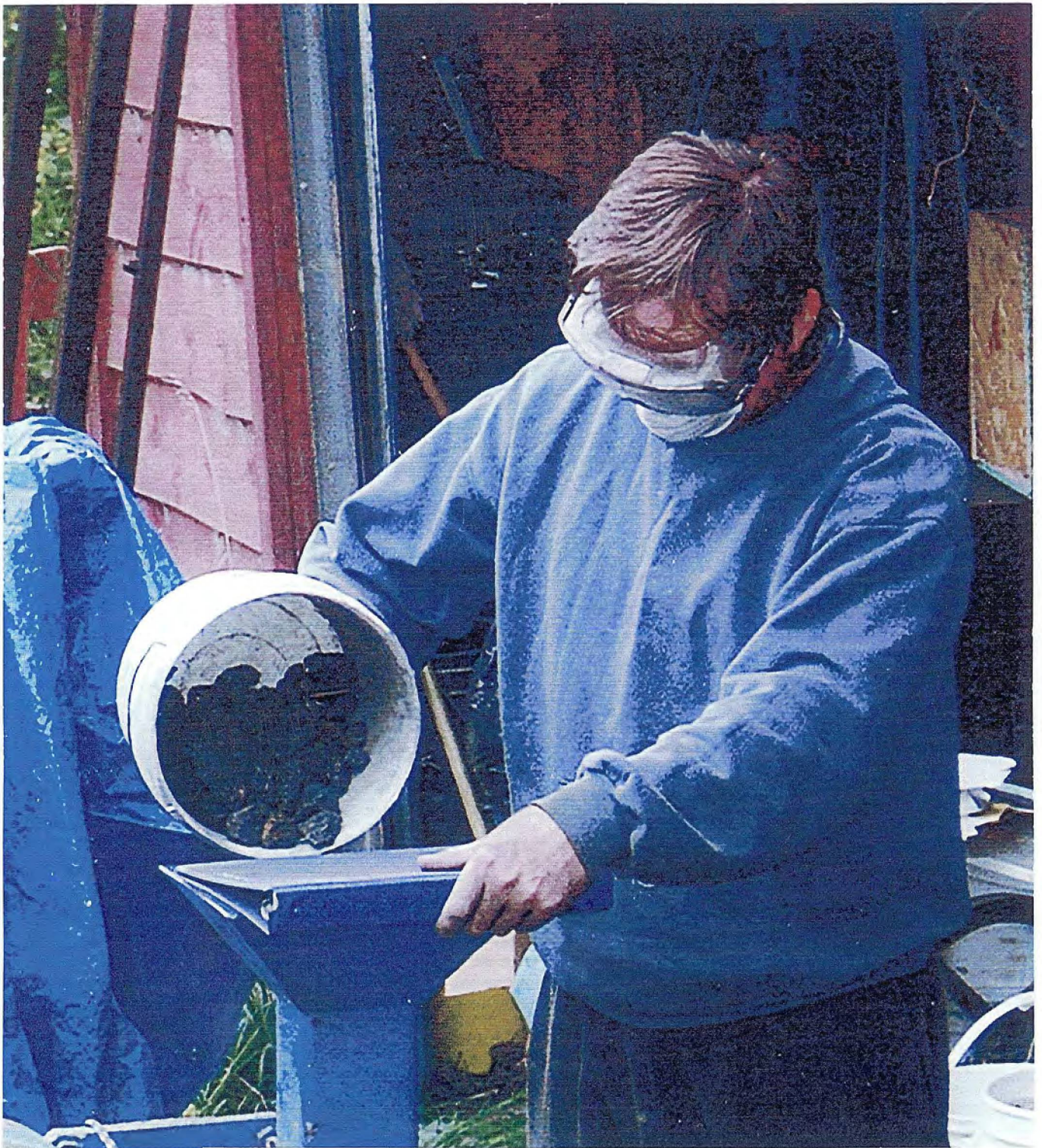
Fig. 4 – Testing an impact crusher on volcanic rock samples
