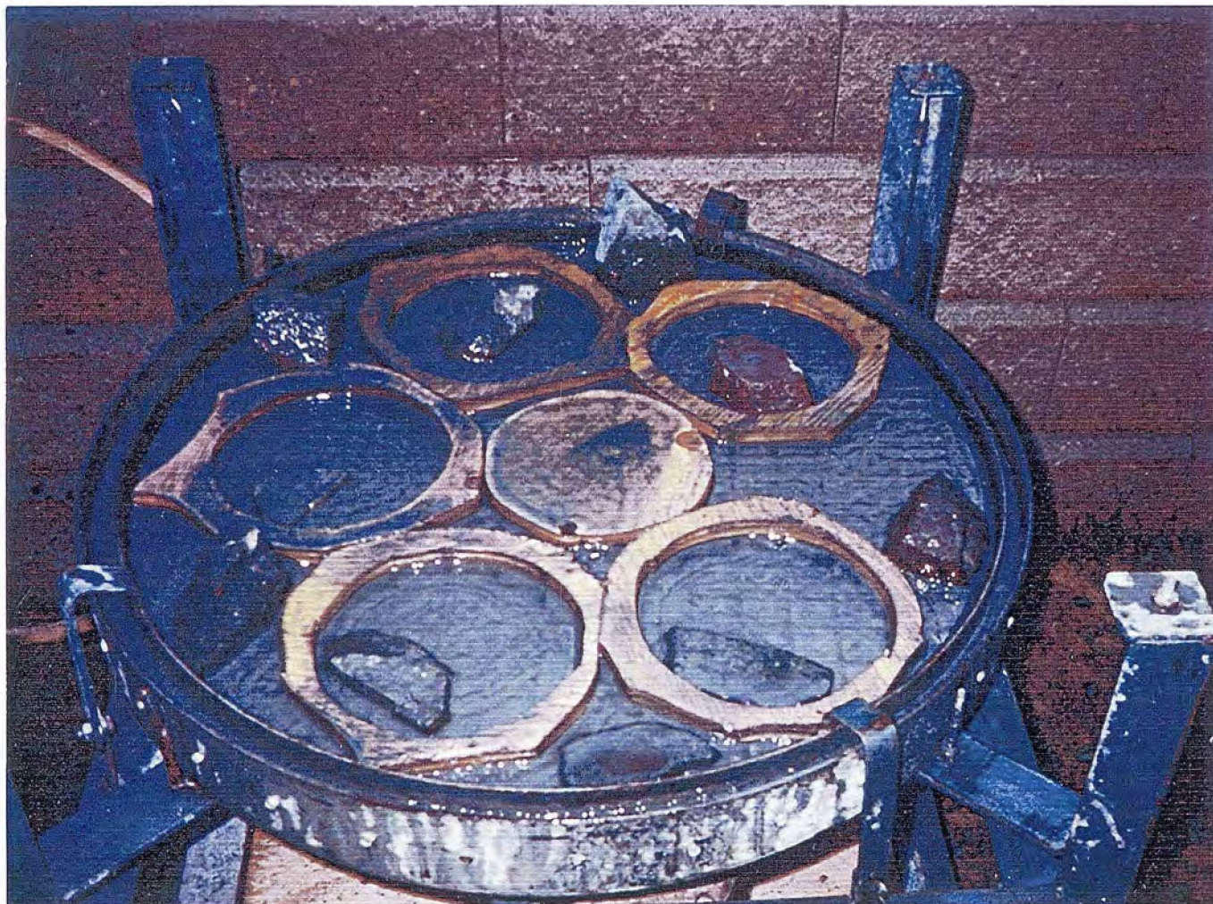
Fig. 7 – Large flat lap machine used to polish rock slabs
