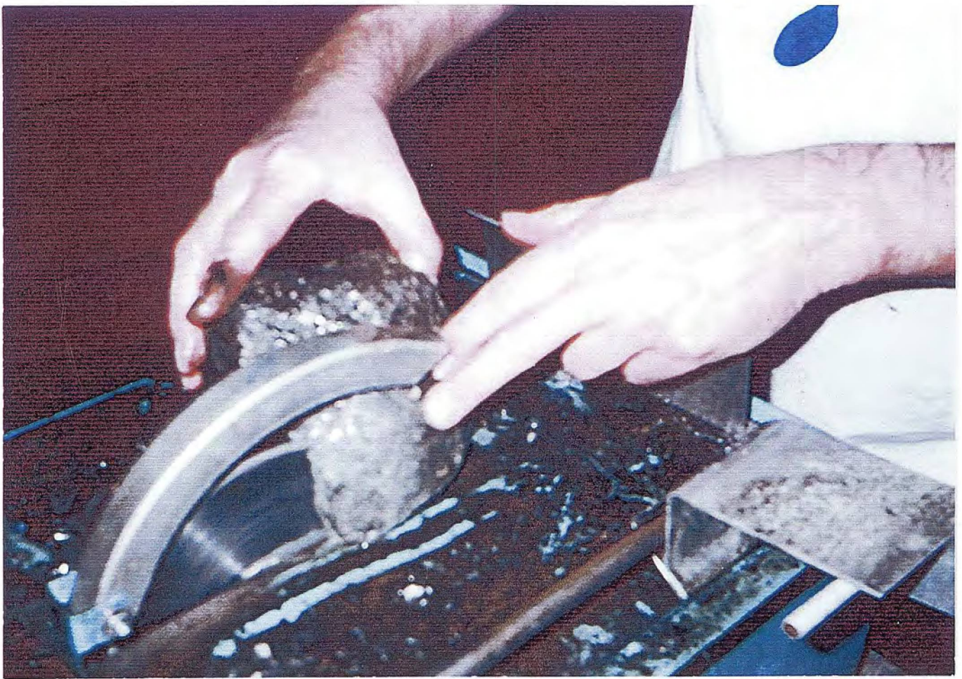
Fig. 5a – Rotary diamond saw cutting slabs
