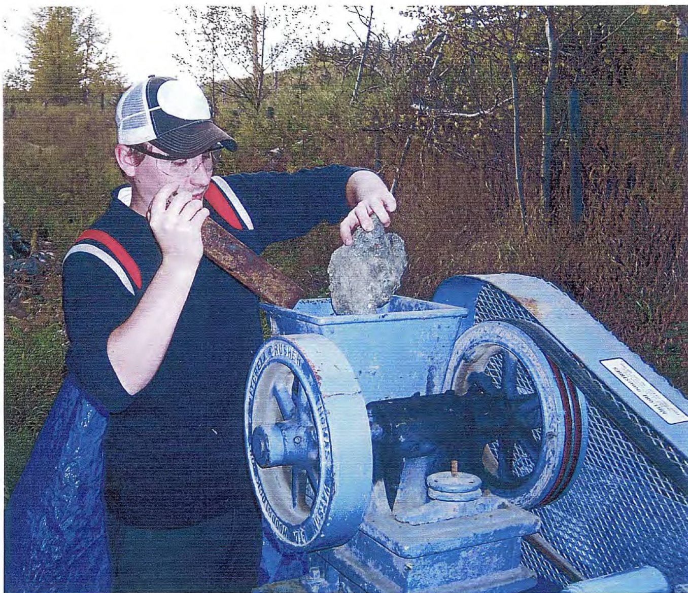
Fig. 3 – Jaw crushing volcanic rock samples
