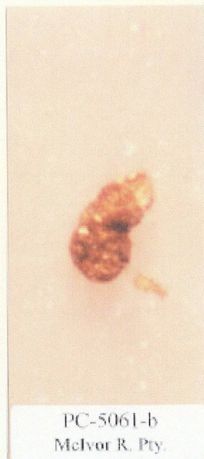
Plate B1.1 Typical coarse gold grains previously recovered from the vicinity of the confluence of the KRC Tributary and McIvor River, Tintina 1994. Distance between dark lines across images is 1mm (where said lines are not visible, longer dimension of photograph equals approximately 1mm).
