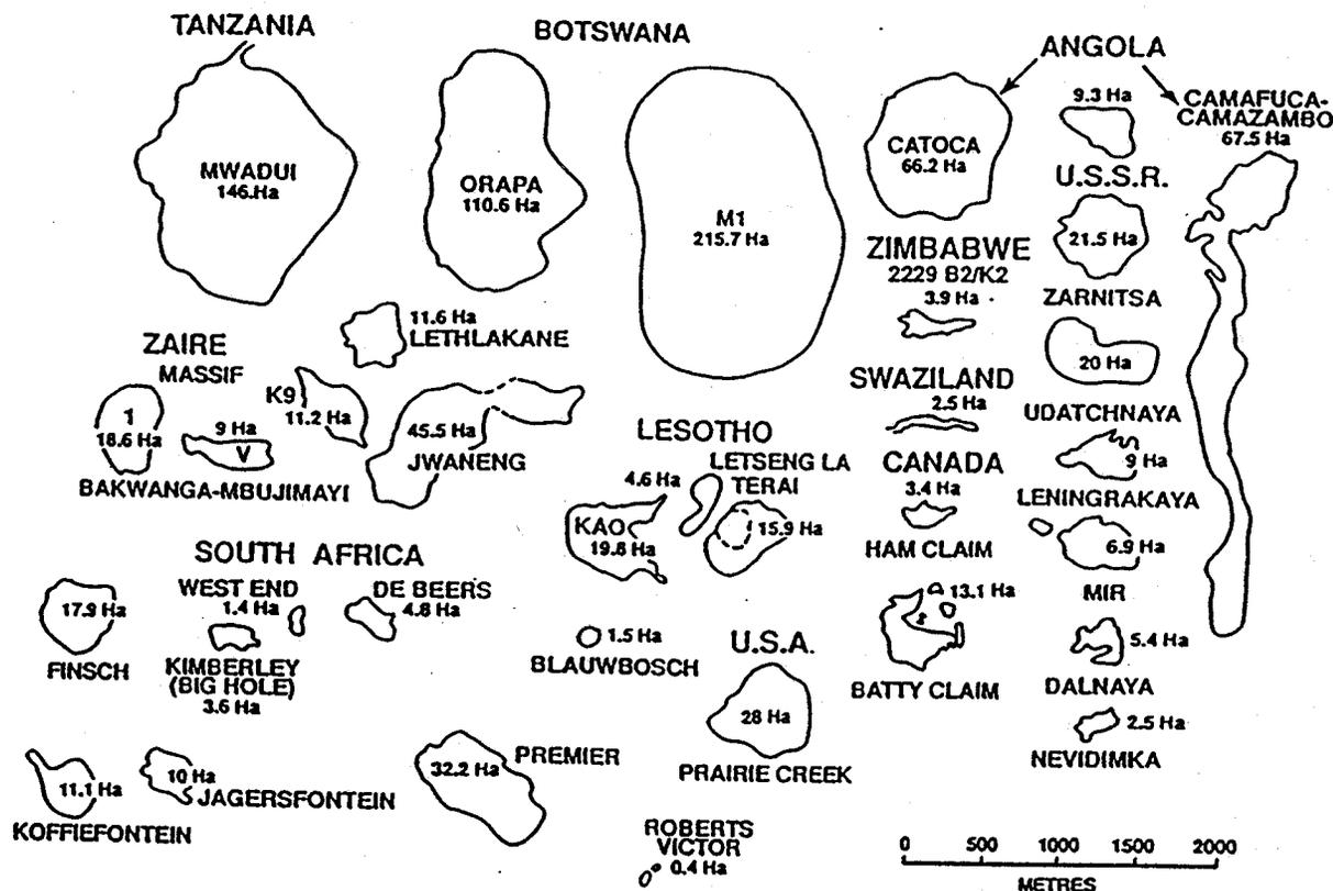
Figure 2 - Shapes and sizes of diamond pipes.
