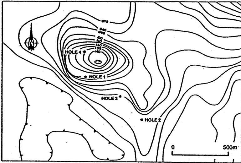
Figure 5 - Ground magnetic survey over a kimberlite pipe.
