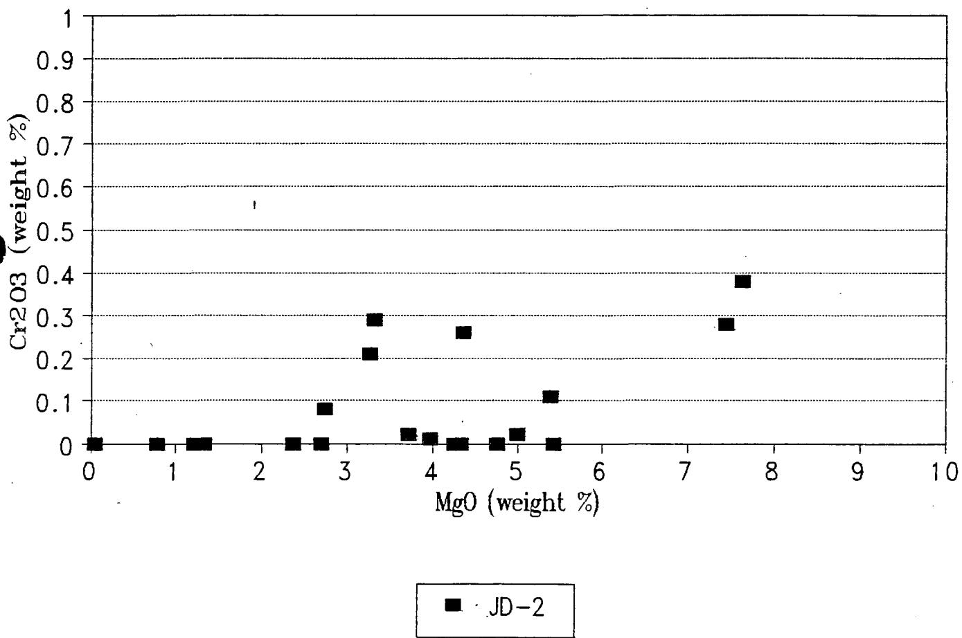
Figure 18 - Cr<sub>2</sub>O<sub>3</sub> vs. MgO graph of ilmenite data determined from grains recovered in southern Alberta. The data shows weak to moderate picroilmenite (MgO) content in the ilmenites analyzed. The six picroilmenite analyses (MgO > 3 wt.%) indicate only moderately reduced conditions, suggesting poor to moderate diamond preservation potential. However, very few ilmenite grains have been analyzed and such interpretations are tenuous at best.
