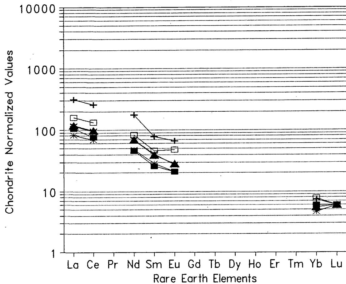
Figure 21 - Plot of REE for southern Alberta intrusive data of Kjarsgaard (1994). Note that the data compares well with the low to intermediate plots of South African kimberlite values (see Figure 23). In addition, note the lack of a Eu anomaly, indicating crystallization depths below feldspar stability.
