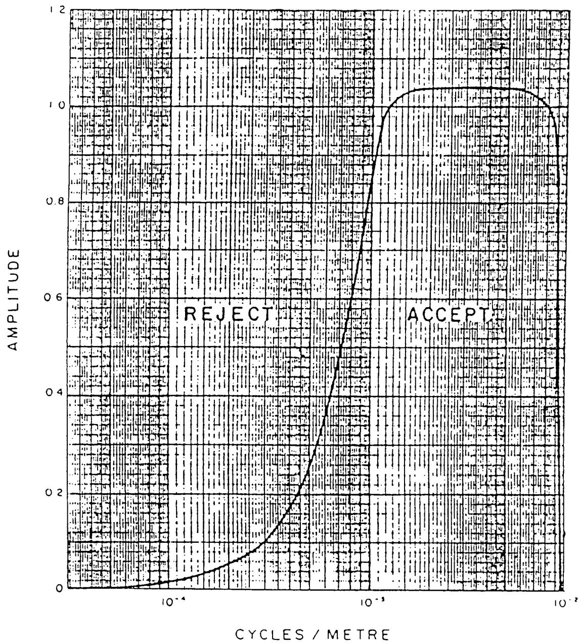
Fig. 5-2 Frequency response of VLF operator.
