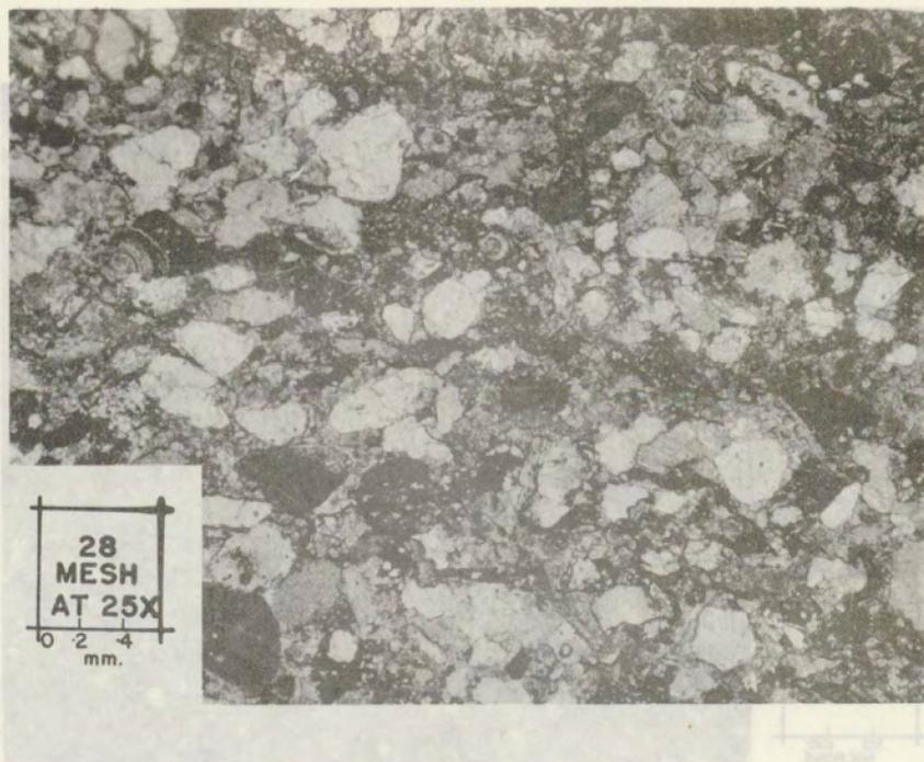
Thin section in plane polarized light, showing relatively large grains of carbonate minerals (white, light grey) and apatite (dark grey to black) in a fine-grained carbonate matrix.
