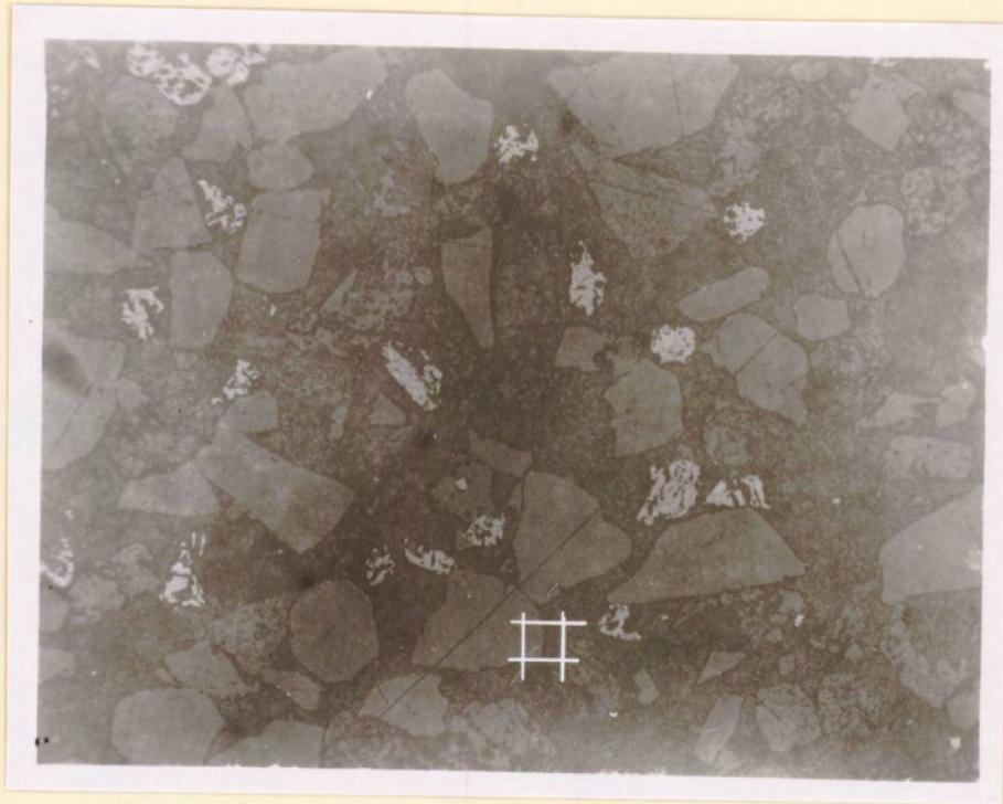
Shows an average field in polished section of sparsely disseminated magnetite (white) in fine carbonate matrix (dark grey rough surface), which also embeds fragments of quartz (medium grey smooth surface); straight black lines are polishing scratches, and white square is a 200-Tyler mesh screen opening.
