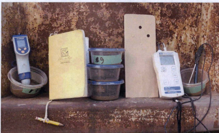
Photograph 2 Soil pH and conductivity measuring equipment
