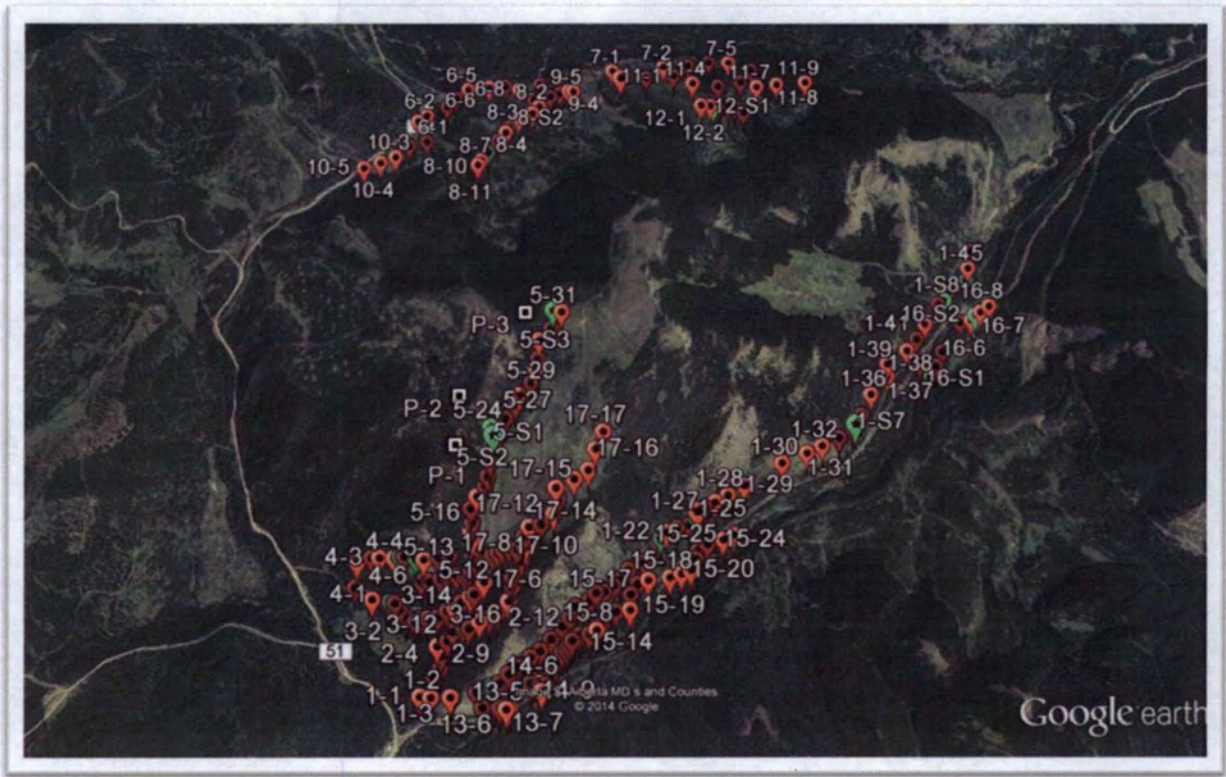
Image of total exploration area with survey line stations and tests pit shown
