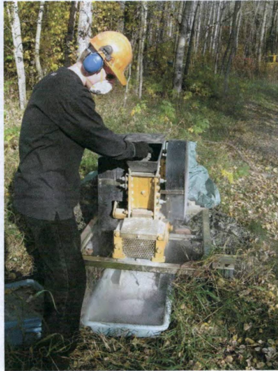
4x6 Jaw over rolls crusher at work
