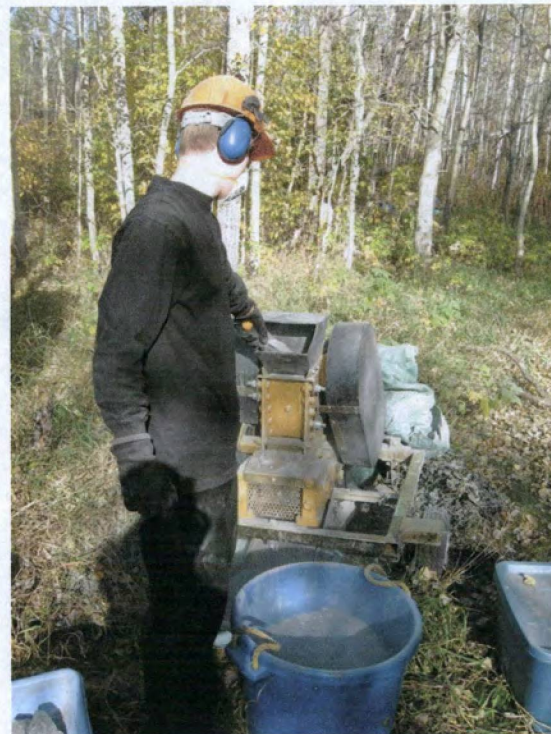
Second pass to produce fine feed for shaker table
