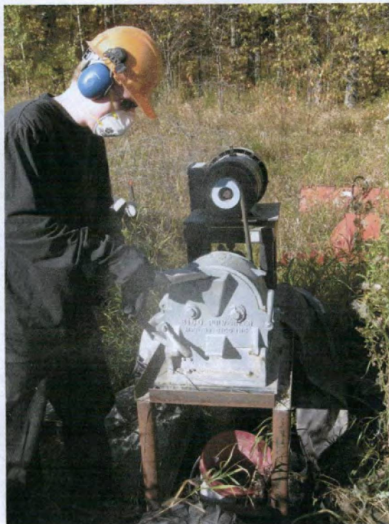
Bico grinder producing consistent minus 120 mesh
