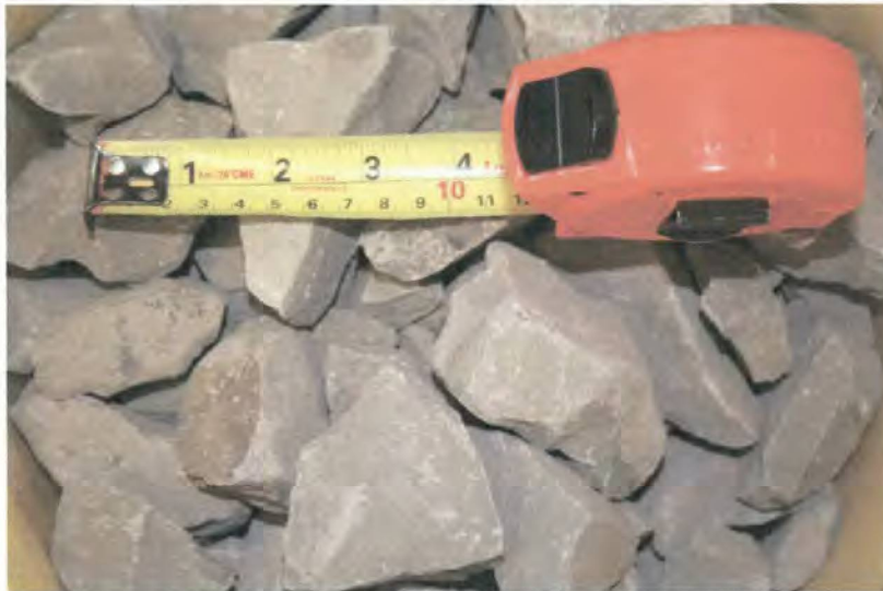
Figure 15 – Crushed and screened sample of Sandstone
