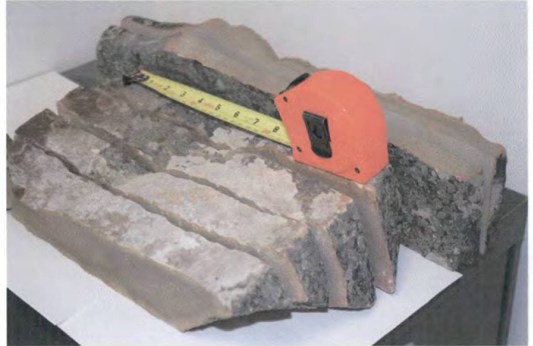
Figure 11a – Thinly Split Sandstone Straight true split regardless of Irregular surface
