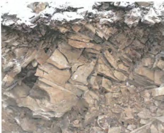
Figure 8 – Test Pit Layered / Fractured Sandstone
