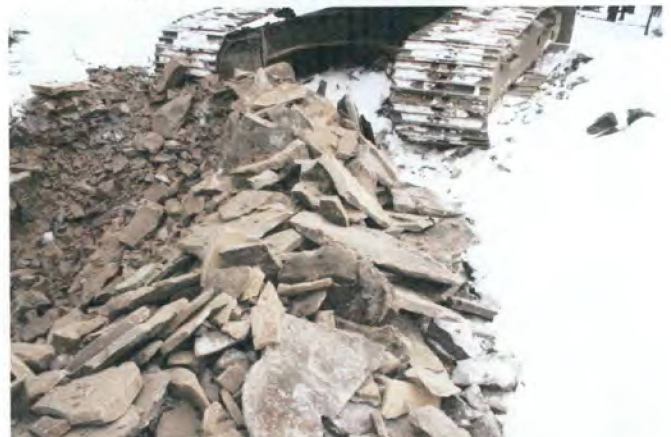
Figure 9 – Thin Flat Layering
