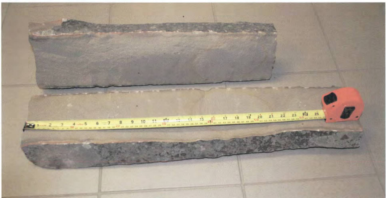
Figure 12 – Excellent Splitting Characteristics – Ideal for masonry applications
