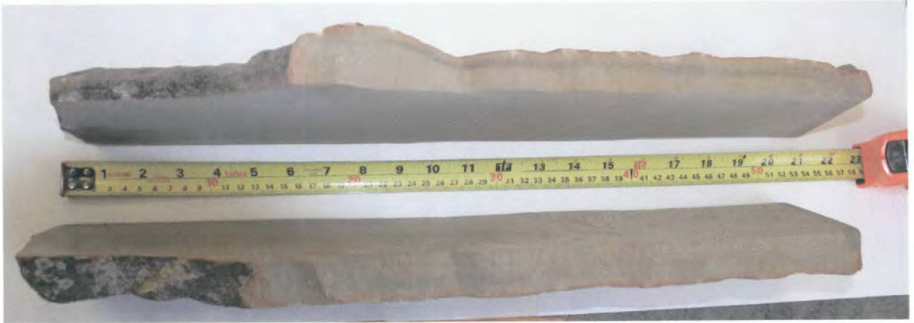
Figure 13 – Saw cut Sandstone Section
