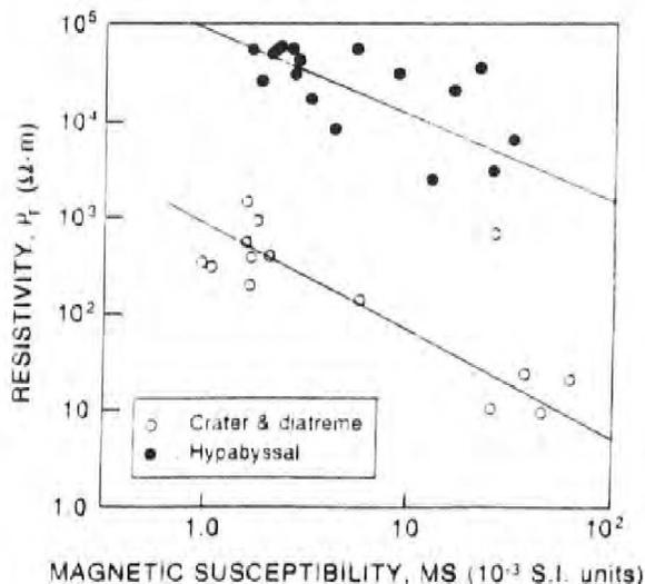
Figure 2: Bulk electrical resistivity ( $\rho_r$ ) as a function of magnetic susceptibility (MS), showing two distinct groups: one for the hypabyssal (HB) kimberlites and the other for the diatreme/crater (DT/CR) kimberlites.
