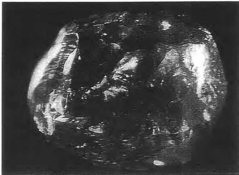
DIAMOND: SIZE L-1.2; W-1.0; T-0.1mm (CLEAVAGE)
