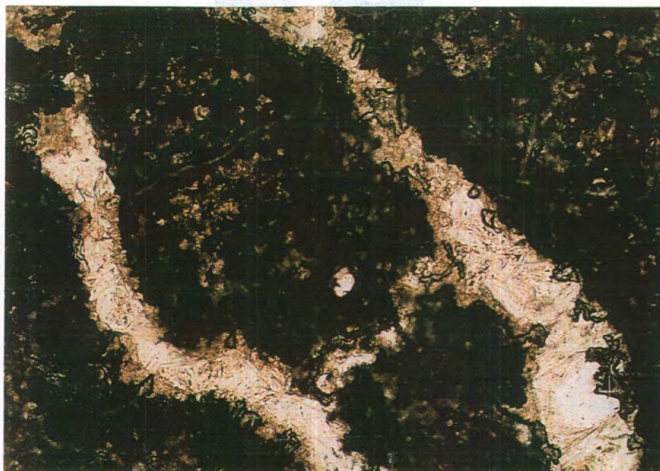
3a high magnification (X100) of fracture infilled by high birefringent low relief fibrous mineral (unidentified) probable calcite or barite but not a zeolite because of the high birefringence
