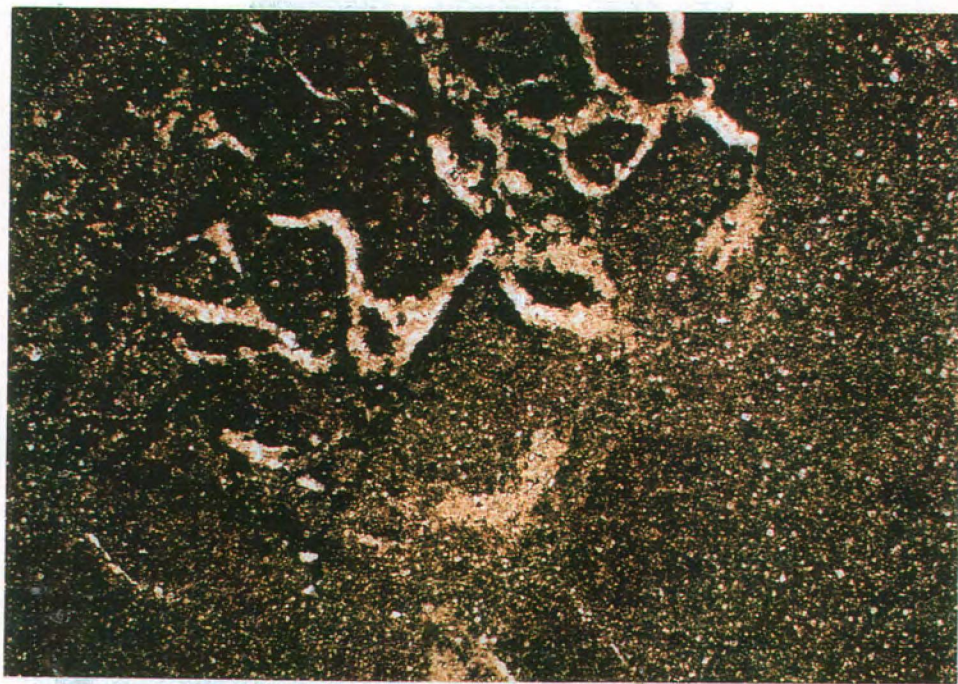
2a general view of a fine textured tuff showing microfractures which give a pseudo-breccia fabric (X20)
