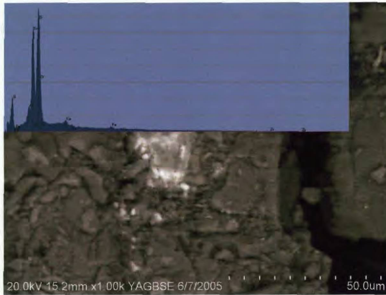
Figure A4 – Backscattered electron image of another region of core 17. The elemental spectrum (inset) is from the zircon-rich bright region.
