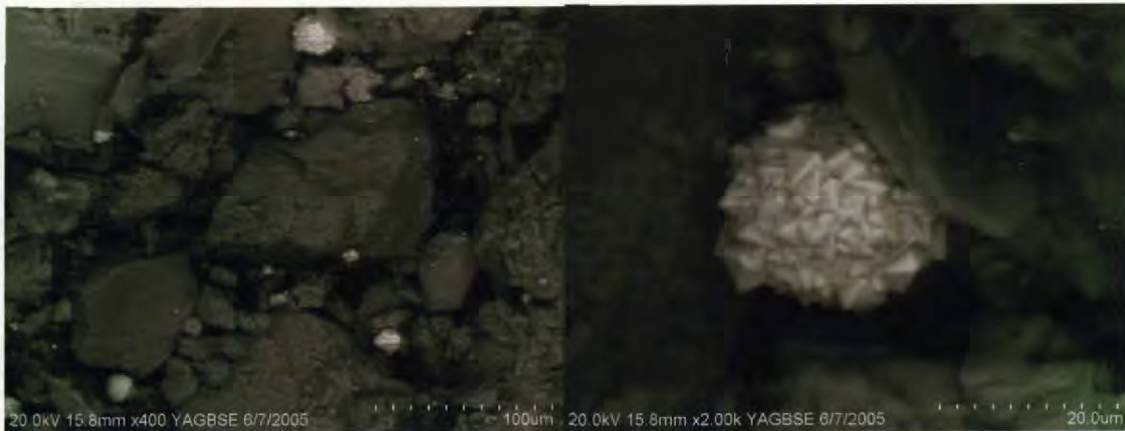
Figure A1 – UTS core #1. SEM image showing the particles with heavy elements brighter than the sand particles. The close-up in the lower micrograph highlights pyrite mineral with framboidal shape.
