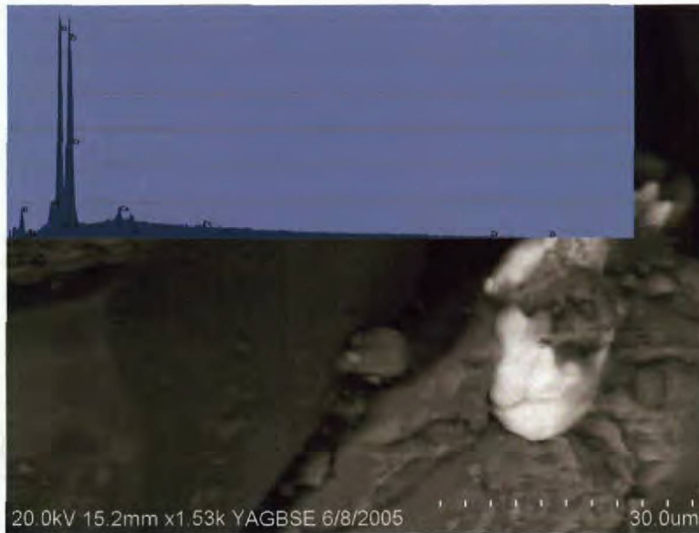
Figure A6 – Backscattered electron image of a region of core 17 rich in heavy minerals. The elemental spectrum (inset) is primarily from the zircon-rich bright region
