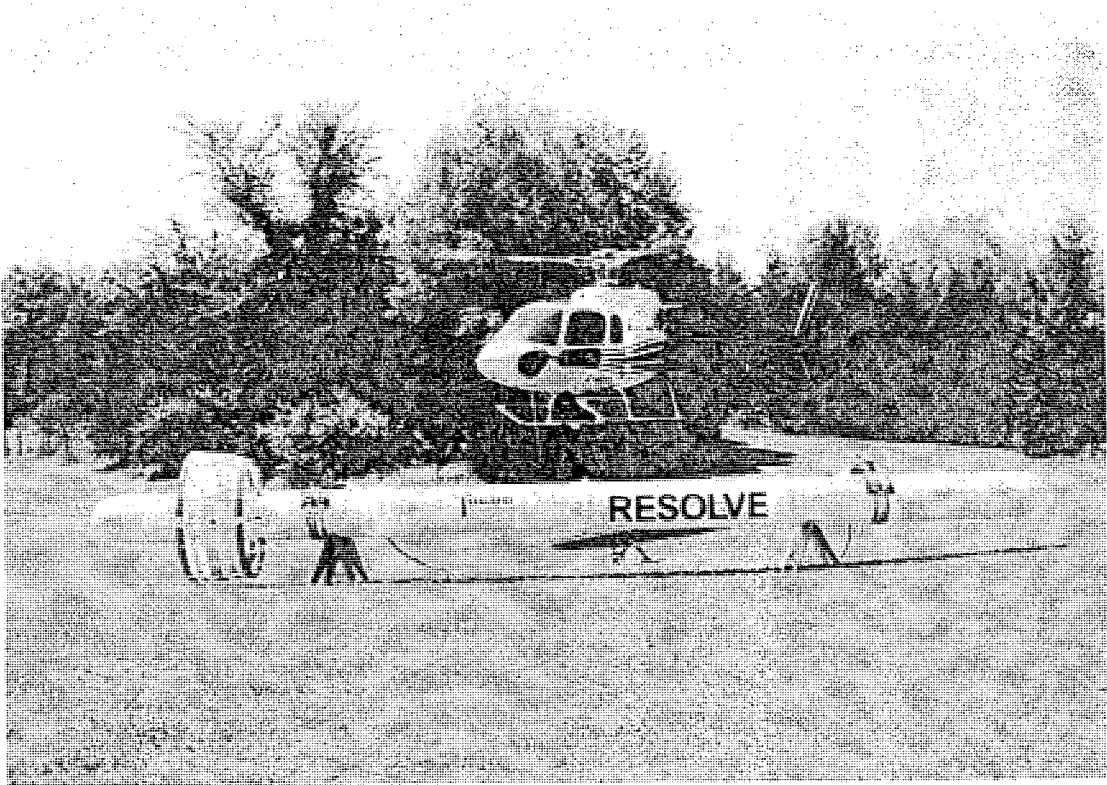
Figure 1: Fugro Airborne Surveys RESOLVE EM bird with AS350-B3
