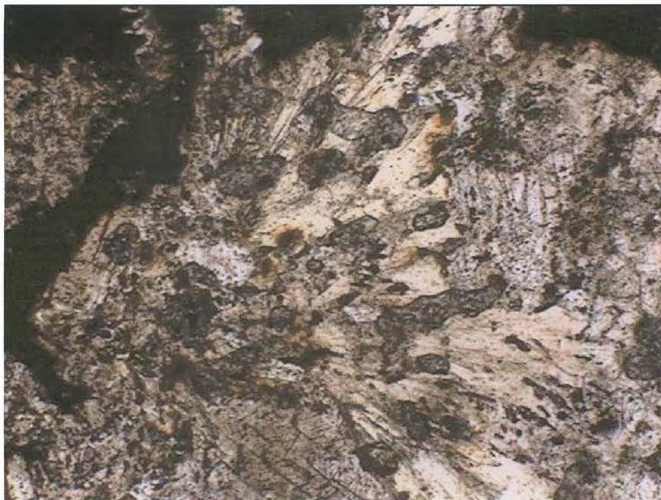
Plate 10/6574: Low magnification view of complex melt/quench texture developed in an irregular quartz/alkali-feldspar grain aggregate. Note strong, fine-grained ornamentation (seen as inclusions) in relic feldspar and quartz. Field of view 1.2x1.0 mm.
