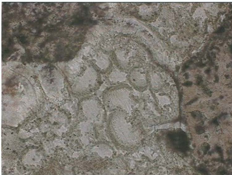
Plate 15/6576: High magnification, plane polarised light view of pseudo-perlitic texture comprising melt/quench textures in quartz grain in granite clast. The greenish-coloured sub-circular structures are interpreted as partially devitrified quench melt. Field of view 1.2x1.0mm.
