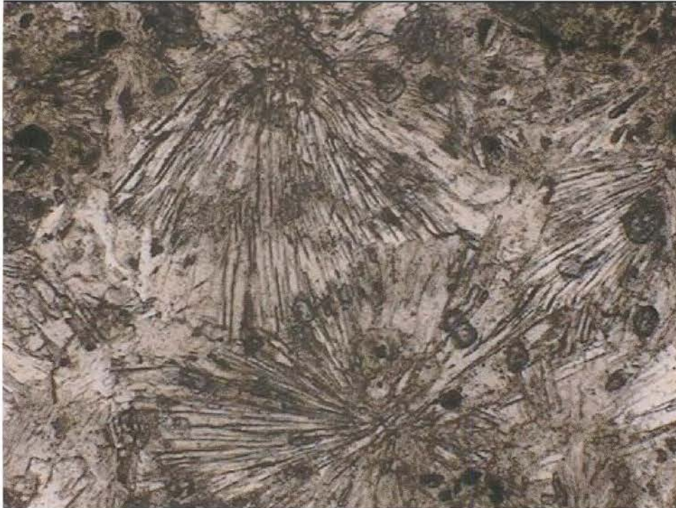
Plate 7/6574: Low magnification view of radial aggregates of quench-textured quartz crystals. Field of view 1.2x1.0 mm.
