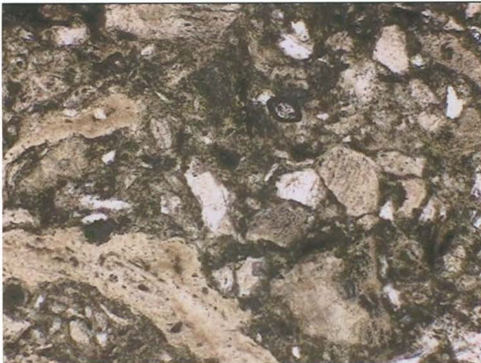
Plate 14/6575: Low magnification view of sample matrix in chaotic micro-breccia. Plate illustrates fluidal-textured felsic fragment, abundant, anhedral quartz grains (clear) and feldspar fragments with distorted cleavage planes. Field of view 1.2x1.0mm.
