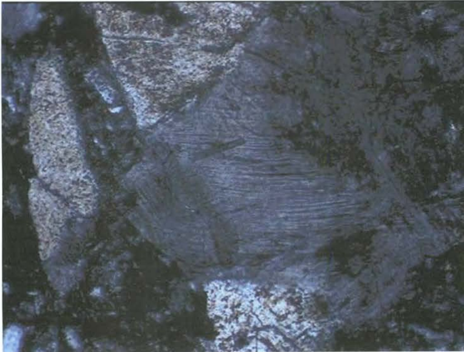
Plate 13/6575: High magnification view of highly distorted cleavage planes in alkali-feldspar. Not strongly decorated quartz grain fragment at bottom-centre of plate. Field of view 0.8x0.65mm.
