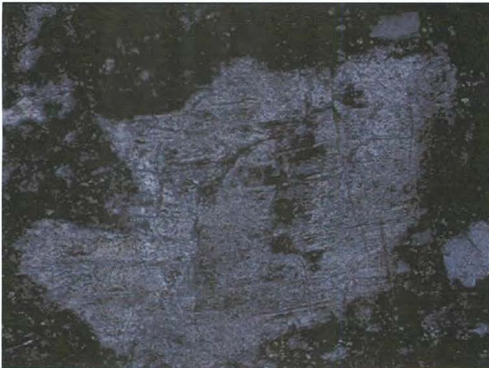
Plate 8/6574: Low magnification view, in crossed-nicols, of distorted cleavage planes in alkali-feldspar crystal. Field of view 1.2x1.0 mm.
