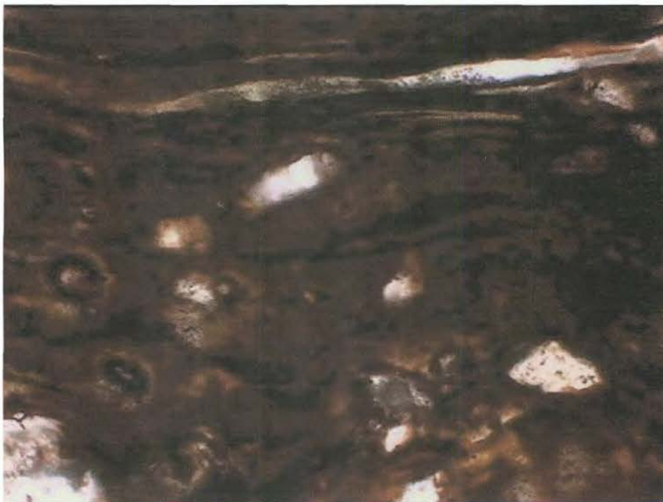
Plate 2/PTS6571: High magnification view of mafic fragment. Note fluidal texture and fine-grained quartz crystal fragments. Field of view 0.8x0.65mm.
