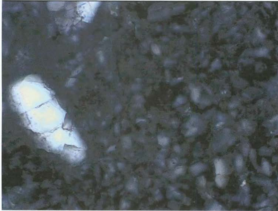
Plate 5/6572: High magnification view, in cross-nicols, of quench texture in mafic fragment and quartz grain fragment inclusion. Field of view 0.8x0.65 mm.
