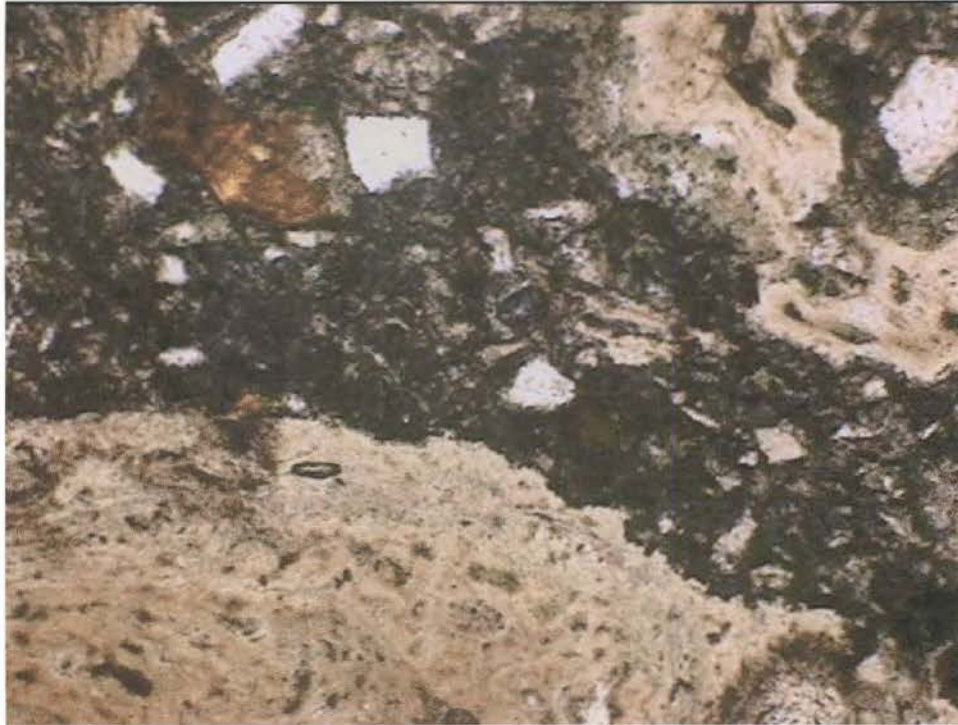
Plate 11/6575: Low magnification view of the contact area between quenched felsic melt and mafic fragment. Note fluidal textural in quench-textured felsic melt and abundance of quartz crystal fragments in matrix. Field of view 1.2x1.0mm.
