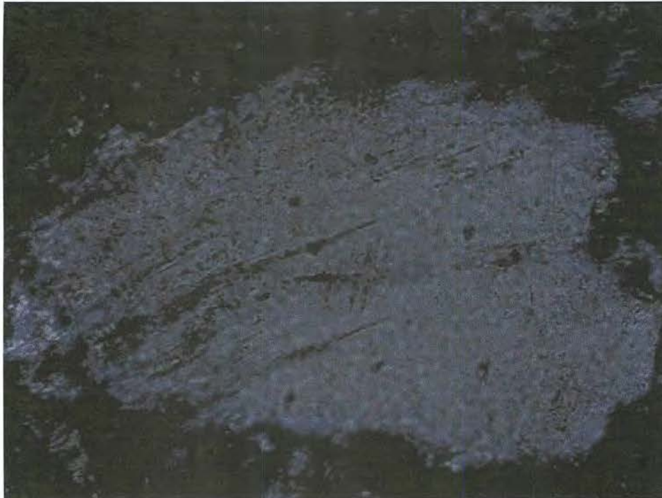
Plate 9/6574: Low magnification view, in crossed-nicols, of distorted deformation lamellae and ornamentation in shocked quartz grain fragment. Field of view 1.2x1.0 mm.
