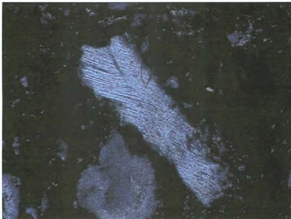
Plate 3/6571: Low magnification view of distorted deformation lamellae in an elongate quartz crystal fragment and rounded melt/quench textures developed in adjacent rounded quartz fragment. Field of view 1.2x1.0 mm.
