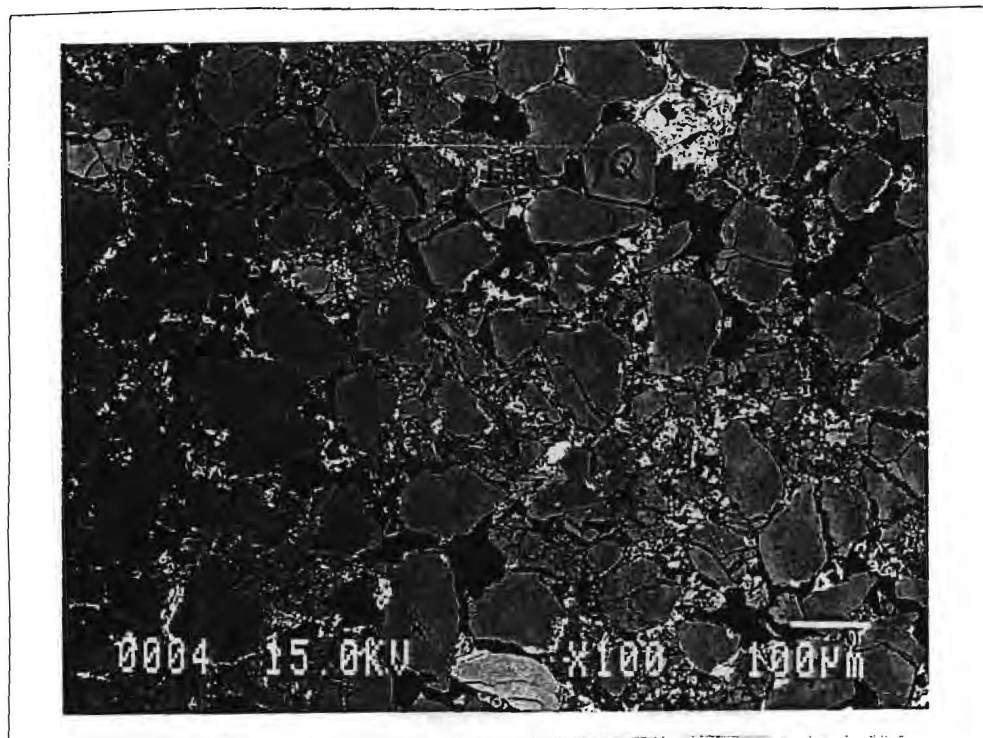
004 detrital quartz grains with lithic grains and isolated biotite and K-feldspar grains; limonite (Fe oxide) in matrix with clay minerals (illite + kaolinite ± chlorite) ± authigenic K-feldspar cement (adularia).
