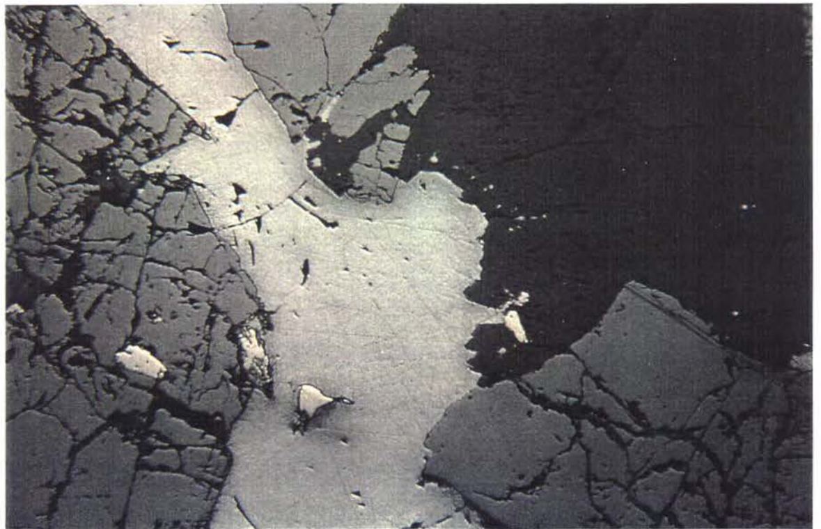
O.R. 97-4 Intergrowth of galena, sphalerite, and ankerite, with minor pyrite. Some fractures in sphalerite are filled with ankerite. Reflected light. Length of photo 2.85 mm.
