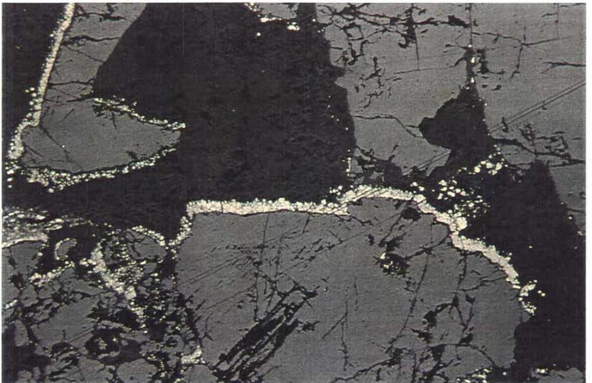
O.R. 97-6 Sphalerite-ankerite intergrowth, seams of cryptocrystalline pyrite on some sphalerite-carbonate grain borders. Reflected light. Length of photo 1.6 mm.
