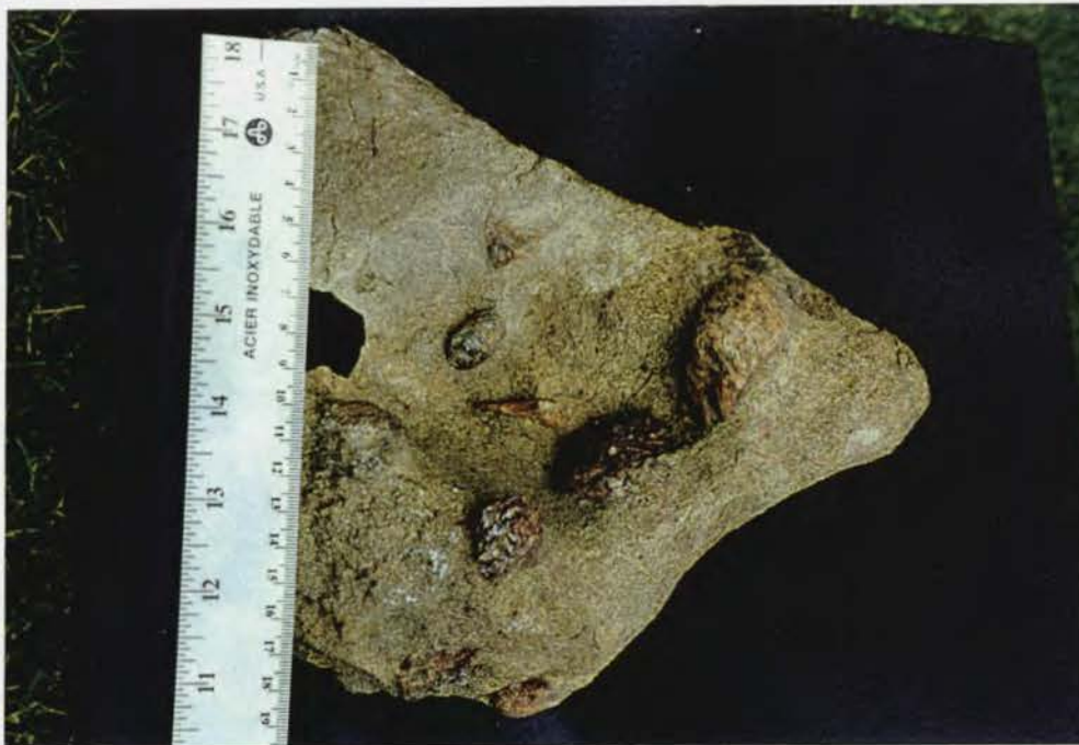
Photo 7: Coarse grained tuff with crustal xenoliths: hand specimen catalogue # 008 Sand sized matrix of crustal minerals supports well rounded (milled) crustal xenoliths. Possible kimberlitic volcanic rock.
