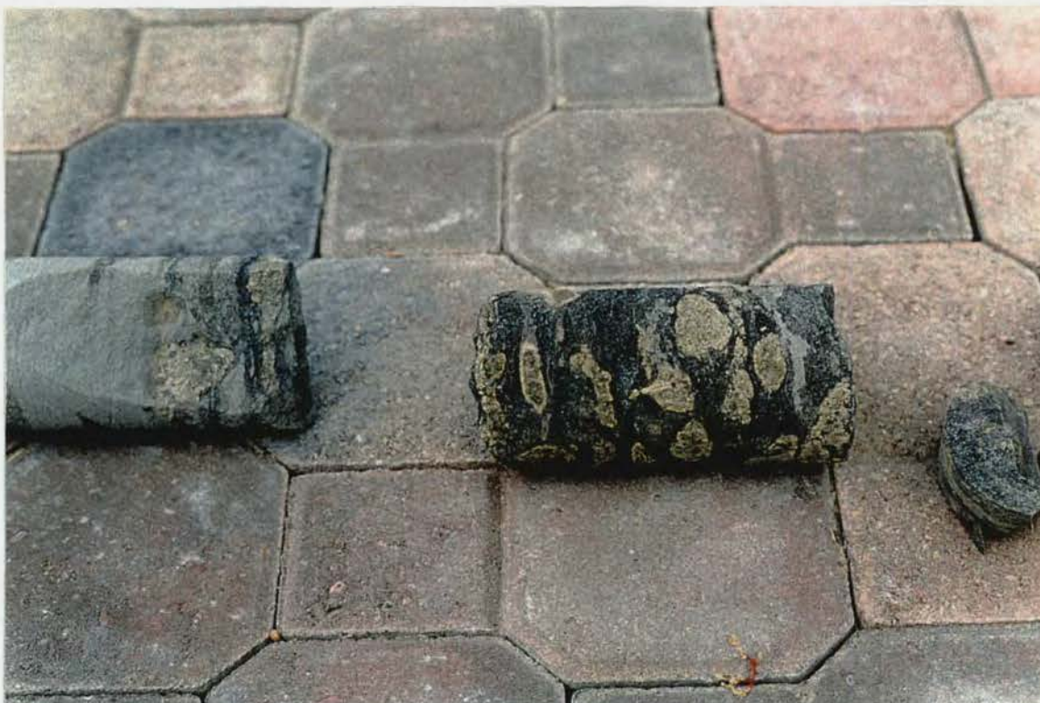
Photo 2: DH 95-1, 332': Glauconitic SS with matrix supported 'clasts'. Clast in section of core at left deforms the sediment underneath it suggesting it was dropped into place.
