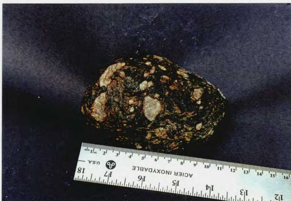
Photo 10: Volcanic breccia: hand specimen catalogue #015. Rolled felsic xenoliths are supported in a fine grained, mafic matrix demonstrating rapid movement of material prior to lithification.
