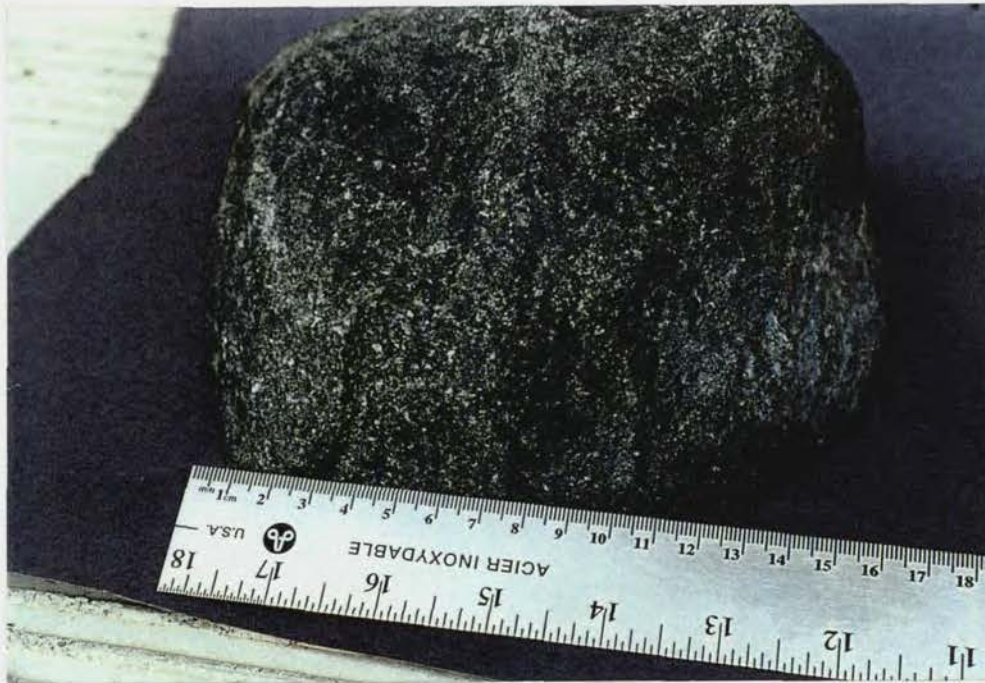
Photo 5: Garnet Pyroxene Gneiss: hand specimen catalogue #001 Probable composition of metabasalt or metagabbro in the eclogite metamorphic facies.
