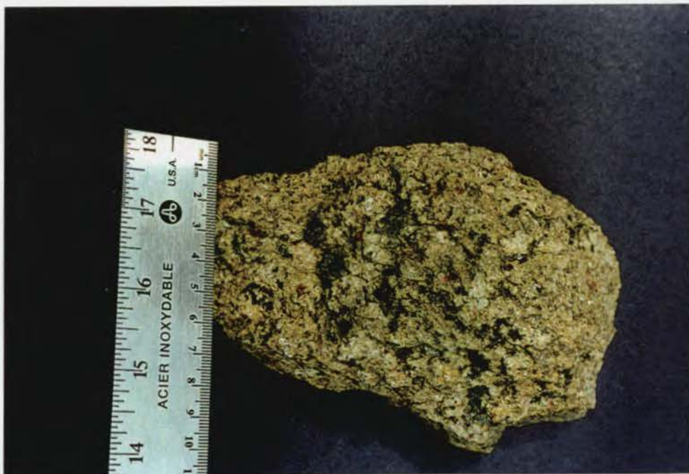
Photo 8: Coarse grained crystal tuff: hand specimen catalogue #016 Mafic and granitic lapilli fragments supported in a matrix of crustal minerals including garnet.
