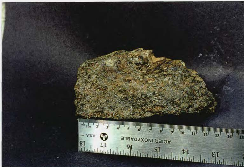
Photo 6: Garnet Pyroxenite: hand specimen catalogue #002 Probable composition of metabasalt or metagabbro in the eclogite metamorphic facies.
