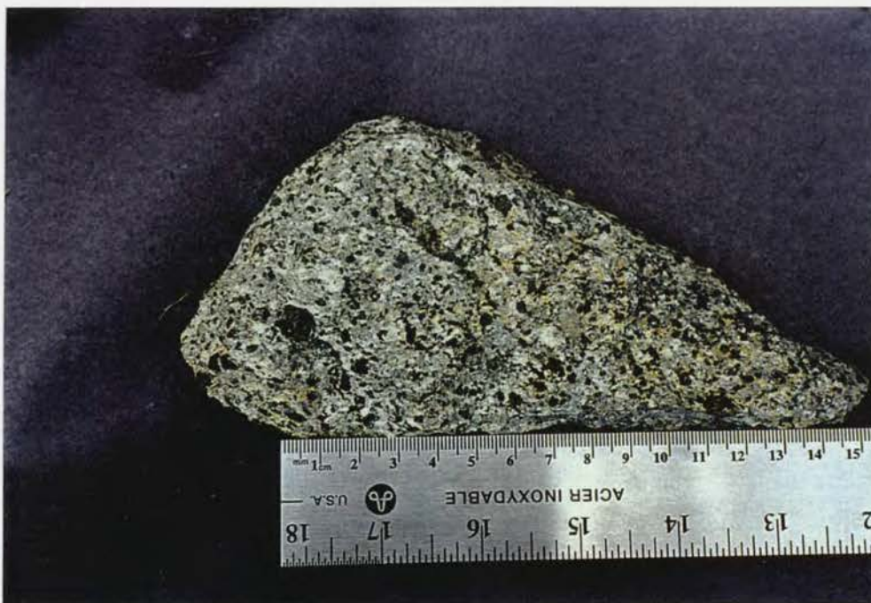
Photo 9: Pyroxene crystal tuff: hand specimen catalogue # 012 Coarse diopside crystals, felsic lapilli and mafic lapilli characterise this sample.
