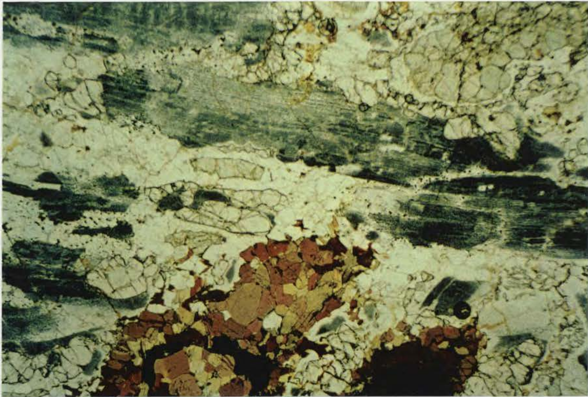
Photo #27: Thin section of hand sample Cat.#003, 32x: granulite facies metamorphism; granular gar., qtz, fsp., bi., amphibole and cpx metamorphically developed at the expense of cloudy plagioclase.
