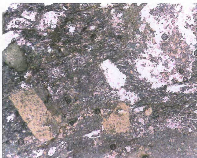
TS.2. x2.5 objective lens altered volcanic rock with amphibole matrix
