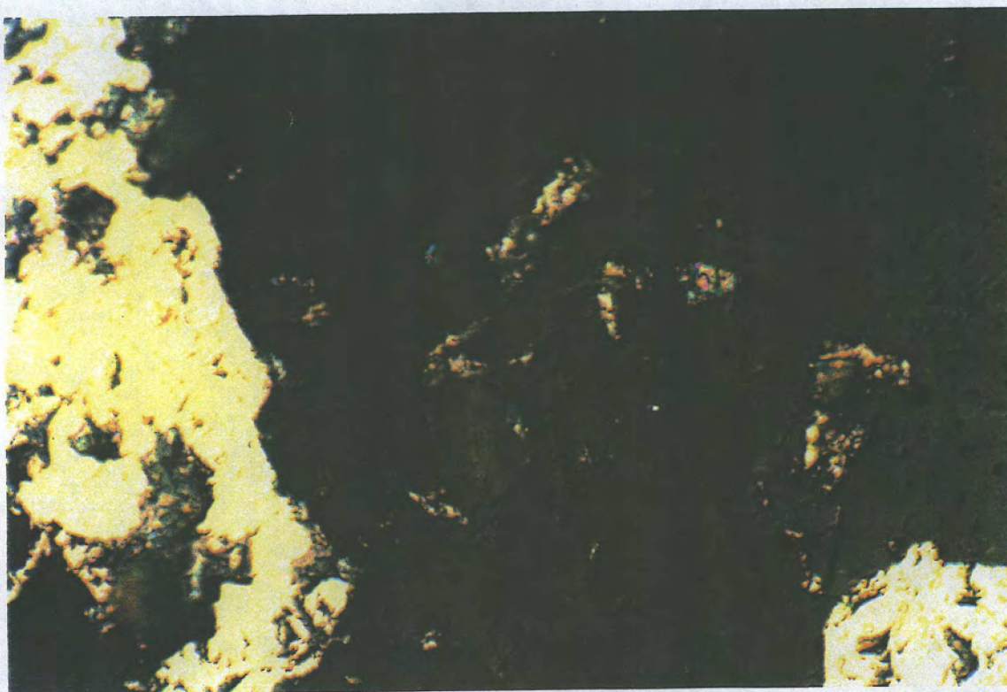
FIG. 18 QT-4 ARSENOPYRITE GRAINS IN QUARTZ
