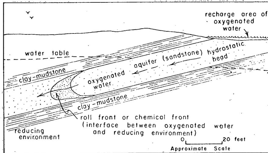
Diag.2 - Schematic cross-section of a sandstone aquifer showing the processes involved in the formation of a roll front orebody (Adler & Sharp, 1967, fig.2)
